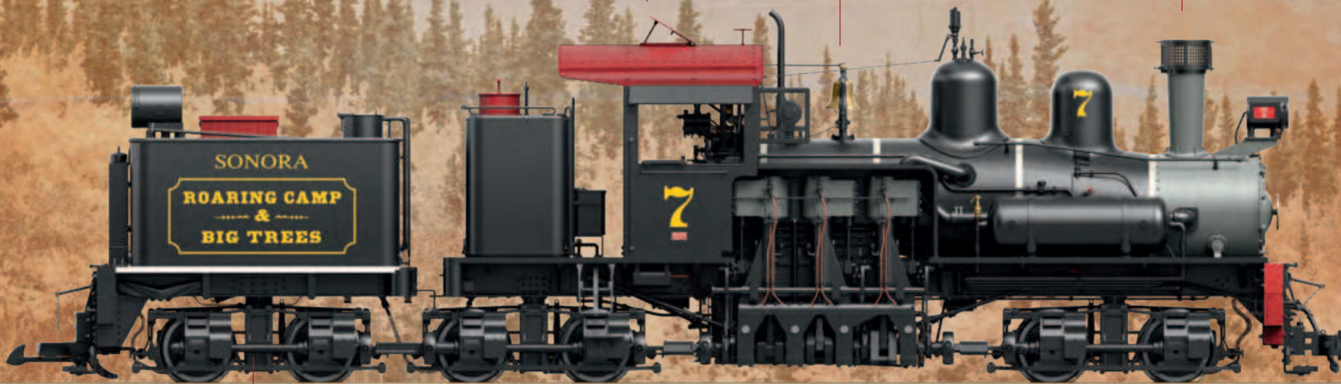
Prototypical drive system using a crankshaft on cardan shafts and rack gears
